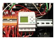
**Programmable Smart Control Automation** provides complete control over the machine's runtime, auto start/stop and timedelay shutdown functionality.
